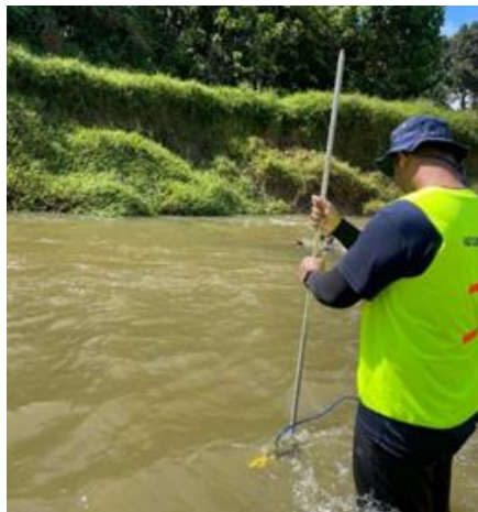
Fig. 4: Wading technique using Current Flow Meter
