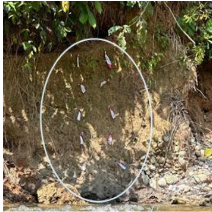
Fig. 3: Erosion pins installed subjected to extreme curve channel after 30 days of installation
