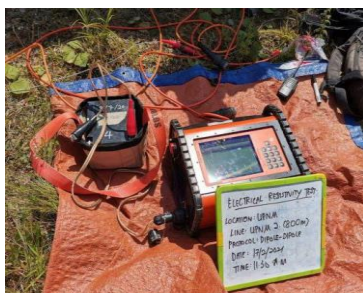
Figure 4. (a) ERT tools employed in this study. (b) Plan view of two ERT traverse lines conducted at site with 400m and 800m length.
