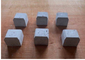
Figure 4: The tilapia fish scale macrocomposite adsorbent.
