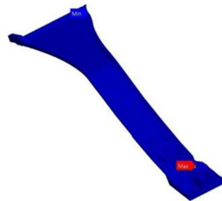
Fig. 37 - Mode shape at 146 m water level
