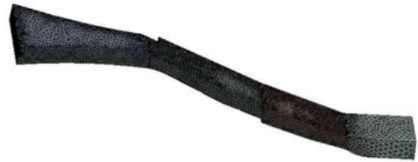
Fig. 5 - Optimum mesh size for spillway fluid section
